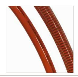
TOUGHJACKET™ hoses have a robust, yet flexible, blended Polyurethane cover extruded directly over the base hose during manufacturing. These hoses are not only sleeker than hoses with a PVC sleeve, they are more durable because the cover is engineered with a proprietary blend of polyurethane to act as an abrasion resistant shield. ToughJacket assemblies are over 180 times more abrasion resistant than assemblies with a PVC sleeve.
